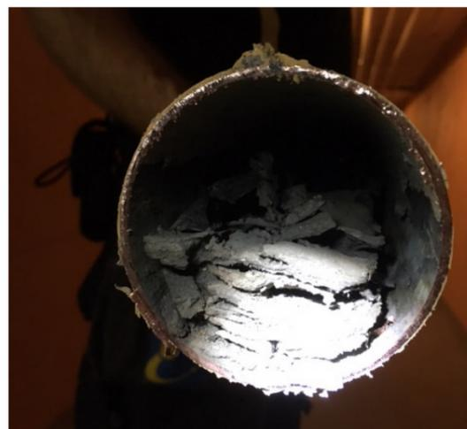
Examples of pipes prior to decontamination
