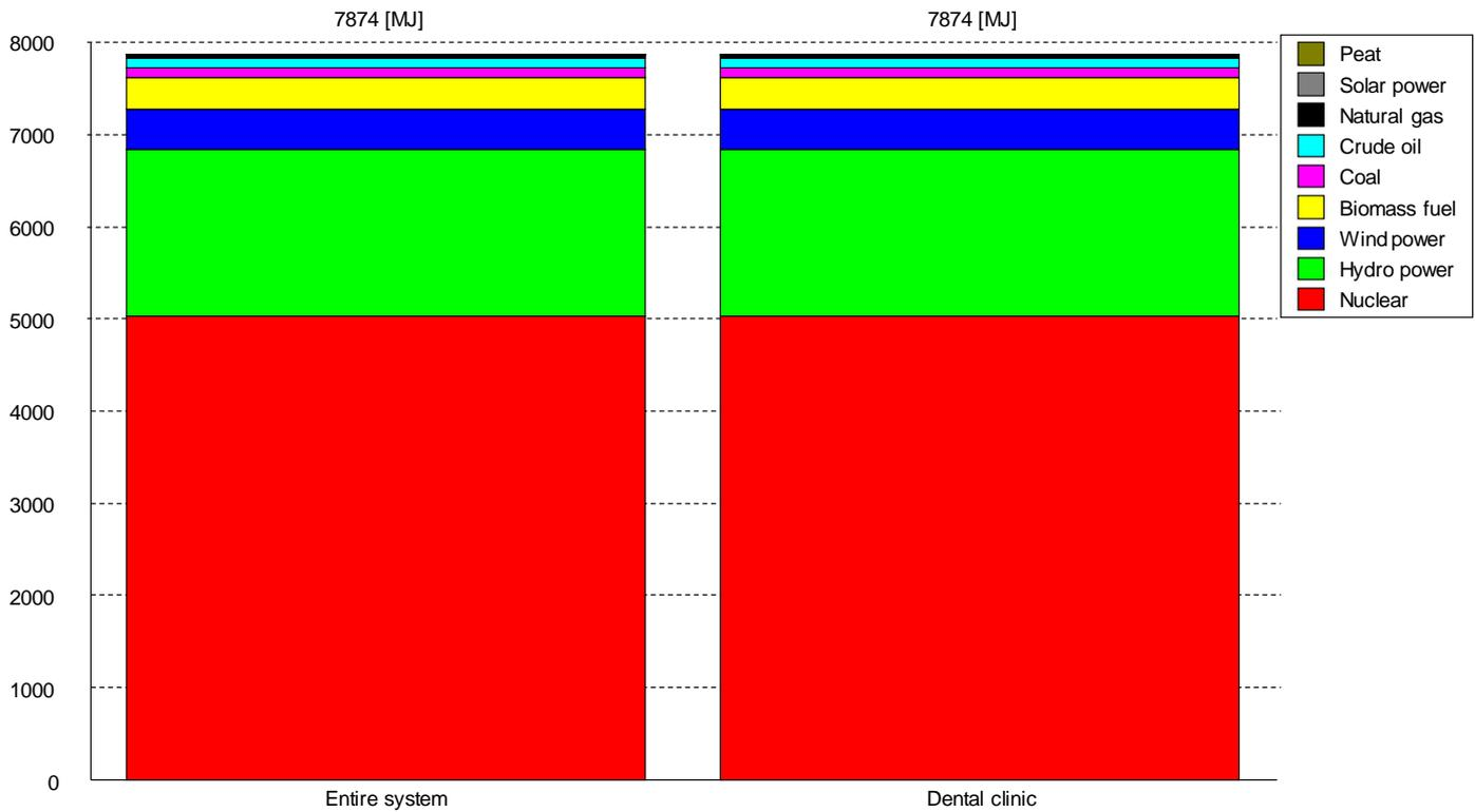
Figure 36 Use of primary energy resources from the entire LCA system including only the Dental clinic without Hg/amalgam separation and expressed in MJ per functional unit. The functional unit is one dentist's chair for one year of operation (226 working days). Scenario 3: with no mercury or amalgam separation or handling, all to recipient.
