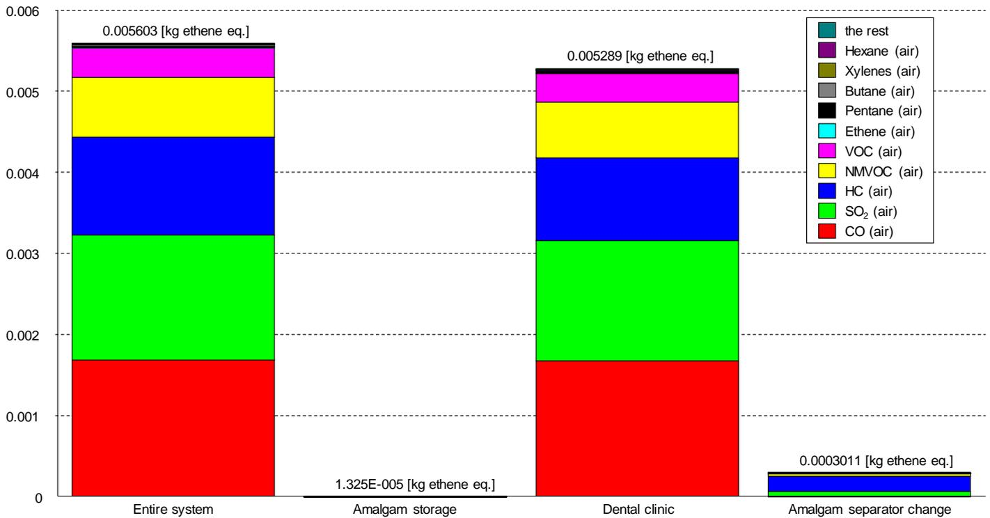
Figure 29 Photochemical ozone creation potentials (POCP) from the entire LCA system and divided in Dental clinic, Amalgam storage, and Amalgam separator change and expressed in kg ethene equivalents per functional unit. The functional unit is one dentist's chair for one year of operation (226 working days). Scenario 2: with only amalgam separation and final storage of amalgam.
