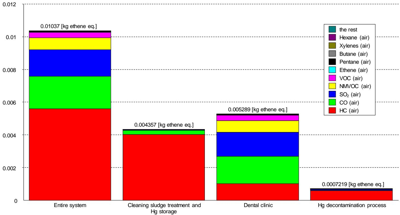
Figure 18 Photochemical ozone creation potentials (POCP) from the entire LCA system and divided in Dental clinic, Cleaning sludge treatment and Hg storage, and Hg decontamination process and expressed in kg ethene equivalents per functional unit. The functional unit is one dentist's chair for one year of operation (226 working days). Scenario 1: with Hg decontamination, Hg processing, and final Hg storage.
