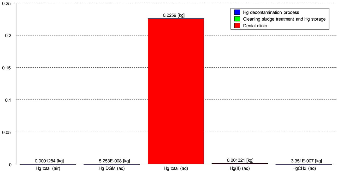
**Figure 35 Total Hg emissions from the entire LCA system expressed in kg per functional unit. The functional unit is one dentist's chair for one year of operation (226 working days). Scenario 3: with no mercury or amalgam separation or handling, all to recipient.**
