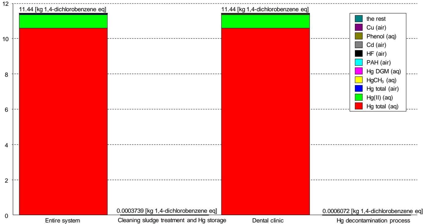
**Figure 22** Freshwater aquatic ecotoxicity values from the entire LCA system and divided in Dental clinic, Cleaning sludge treatment and Hg storage, and Hg decontamination process and expressed in kg 1,4-dichlorobenzene equivalents per functional unit. The functional unit is one dentist's chair for one year of operation (226 working days). Scenario 1: with Hg decontamination, Hg processing, and final Hg storage.
