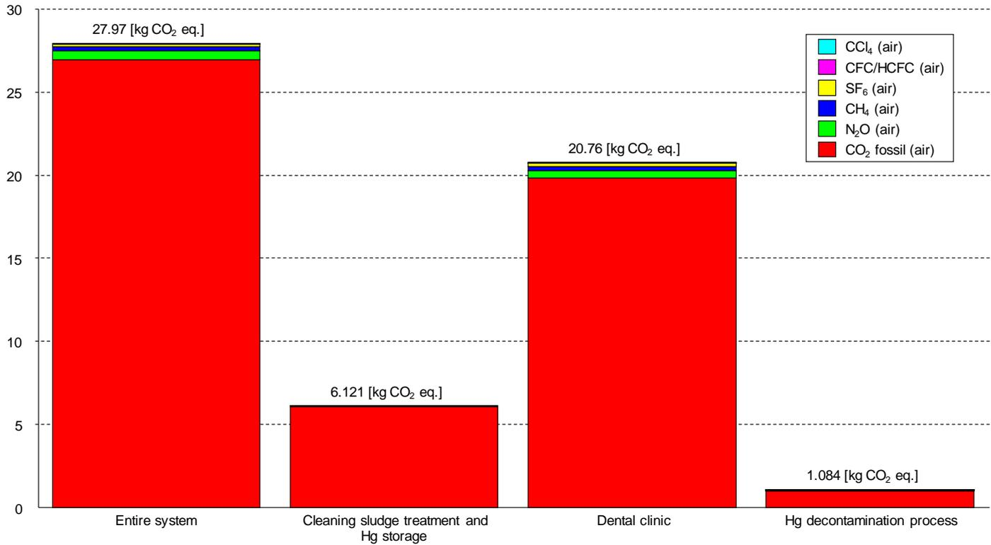
Figure 15 Global warming potential (GWP 100) from the entire LCA system and divided in Dental clinic, Cleaning sludge treatment and Hg storage, and Hg decontamination process and expressed in kg CO<sub>2</sub> equivalents per functional unit. The functional unit is one dentist's chair for one year of operation (226 working days). Scenario 1: with Hg decontamination, Hg processing, and final Hg storage.
