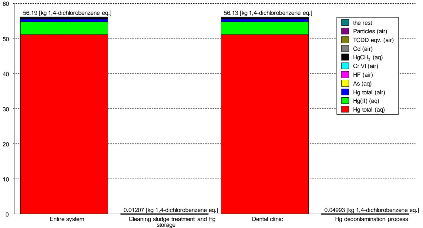
Figure 19 Human toxicity values from the entire LCA system and divided in Dental clinic, Cleaning sludge treatment and Hg storage, and Hg decontamination process and expressed in kg 1,4-dichlorobenzene equivalents per functional unit. The functional unit is one dentist's chair for one year of operation (226 working days). Scenario 1: with Hg decontamination, Hg processing, and final Hg storage.
