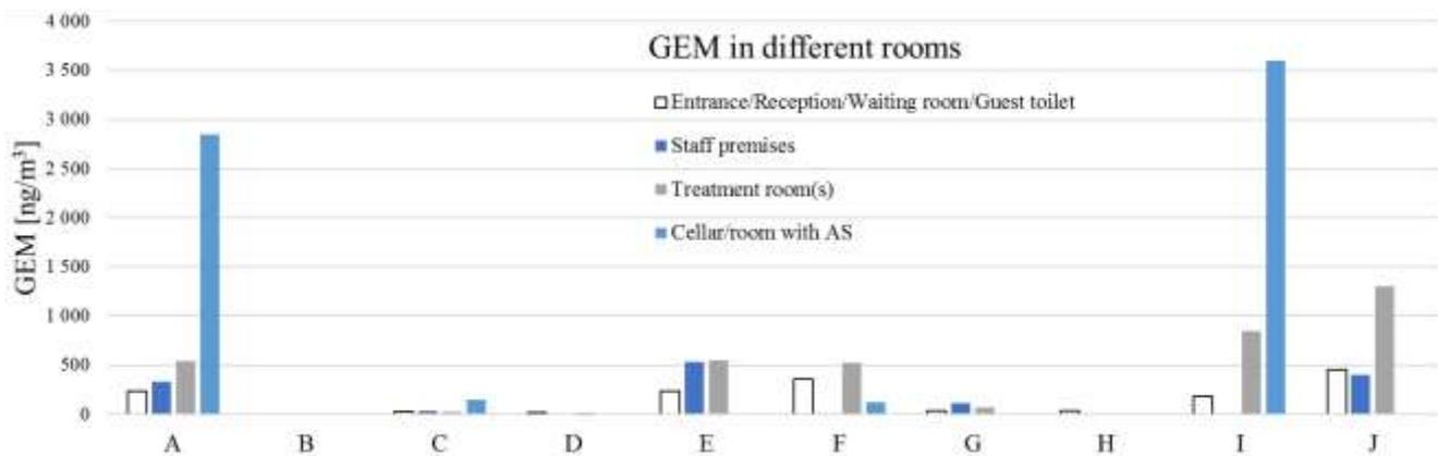
**Figure 5** Average GEM (gaseous elemental mercury) concentrations in air measured at dental clinics A-J in different rooms of the premises before decontamination activities (DC). AS=Amalgam Separator.
