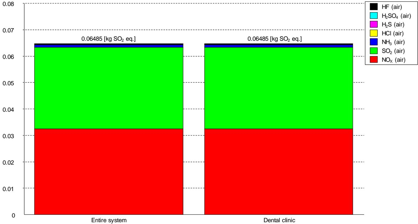
**Figure 39** Acidification potential (AP) from the entire LCA system including only the Dental clinic without Hg/amalgam separation and expressed in kg SO<sub>2</sub> equivalents per functional unit. The functional unit is one dentist's chair for one year of operation (226 working days). Scenario 3: with no mercury or amalgam separation or handling, all to recipient.
