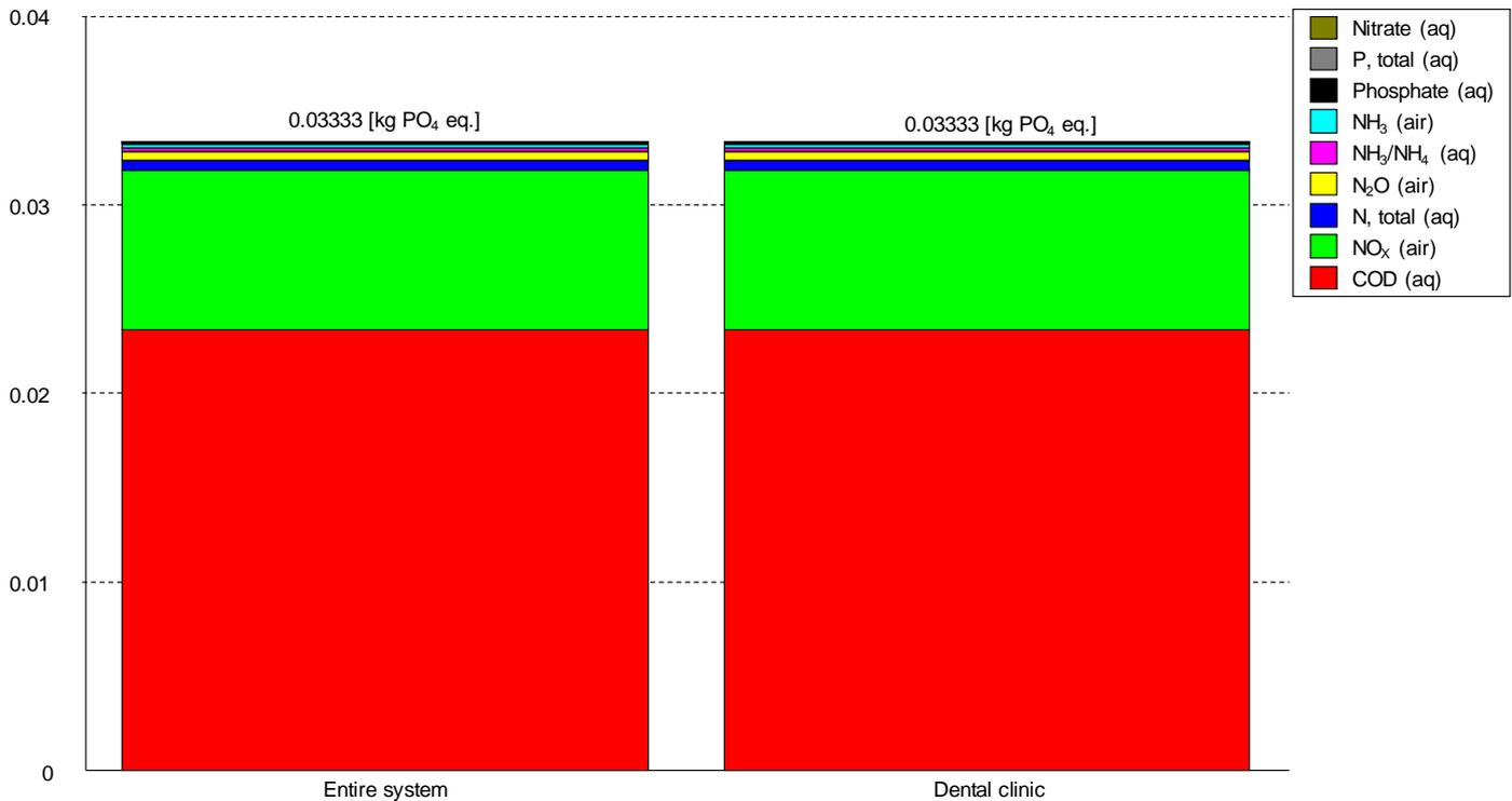
**Figure 38** Eutrophication potential (EP) from the entire LCA system including only the Dental clinic without Hg/amalgam separation and expressed in kg PO<sub>4</sub><sup>3-</sup> equivalents per functional unit. The functional unit is one dentist's chair for one year of operation (226 working days). Scenario 3: with no mercury or amalgam separation or handling, all to recipient.
