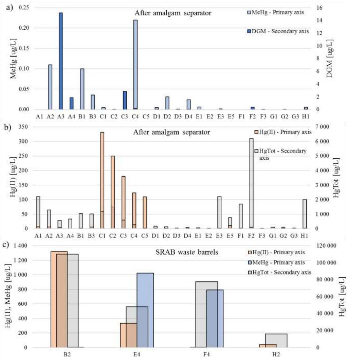
**Figure 8** Analysis results of the 30 samples (Table 2) taken and analyzed by IVL. Samples were analyzed for dissolved gaseous mercury (DGM), oxidized mercury (Hg(II)), methylated mercury (MeHg) and total mercury (HgTot, secondary axis). In a) and b) the results of the samples taken after the amalgam separator (AS) are presented, in c) the samples taken by SRAB from the waste barrels and analyzed by IVL are presented.
