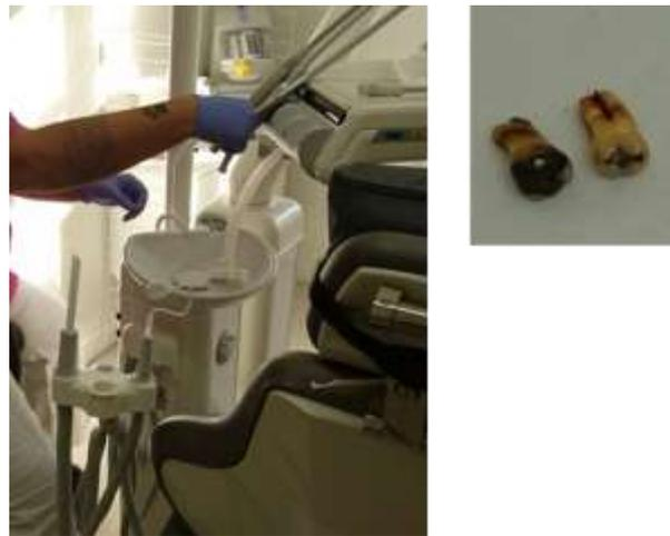
**Figure 10** Test setup of drilling in an amalgam filling in an extracted tooth at a dental clinic.
