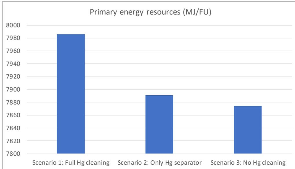
**Figure 48 Scenario comparison of the use of primary energy resources for the entire LCA model systems.**
