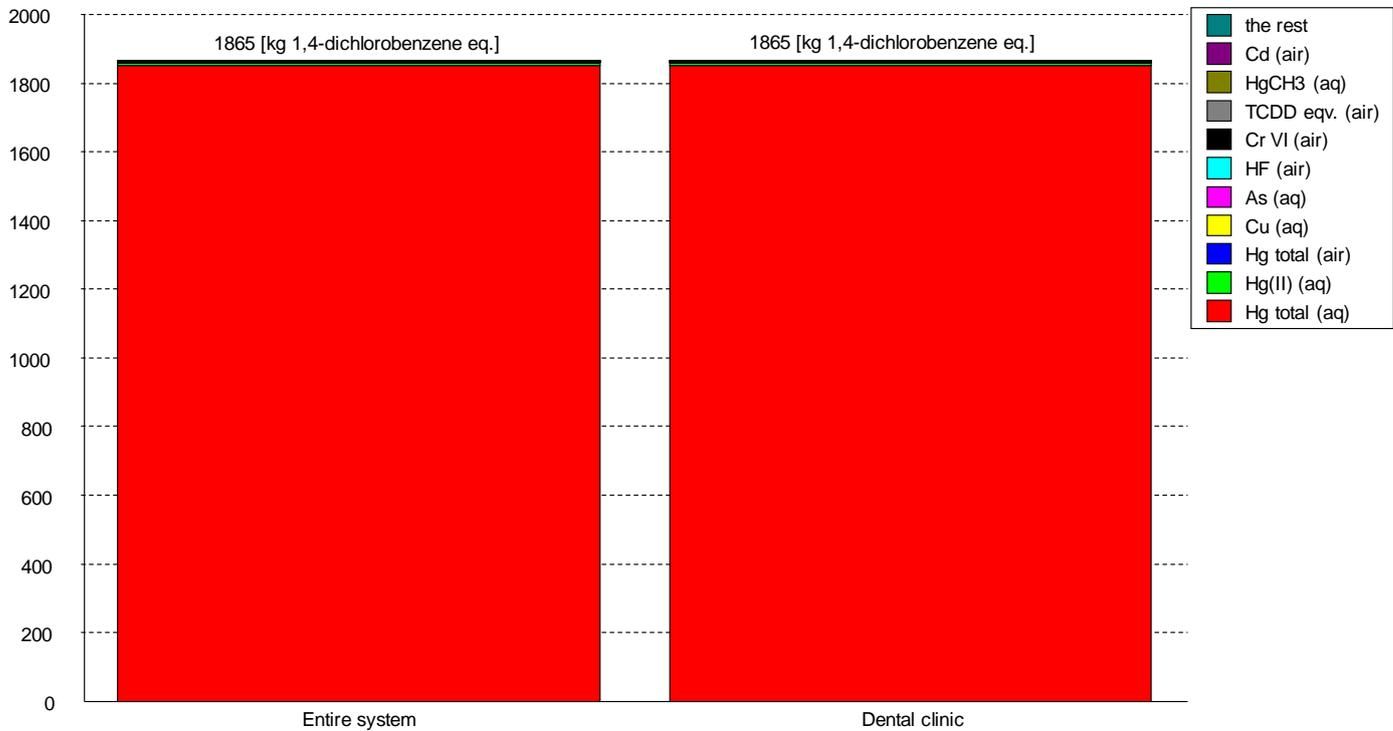
Figure 41 Human toxicity values from the entire LCA system including only the Dental clinic without Hg/amalgam separation and expressed in kg 1,4-dichlorobenzene equivalents per functional unit. The functional unit is one dentist's chair for one year of operation (226 working days). Scenario 3: with no mercury or amalgam separation or handling, all to recipient.
