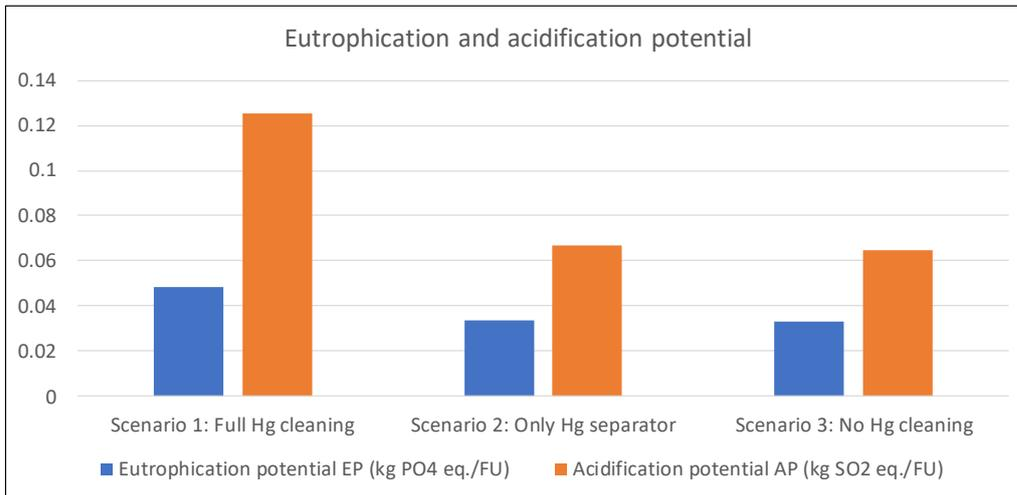
**Figure 50 Scenario comparison of the eutrophication and acidification potential for the entire LCA model systems.**
