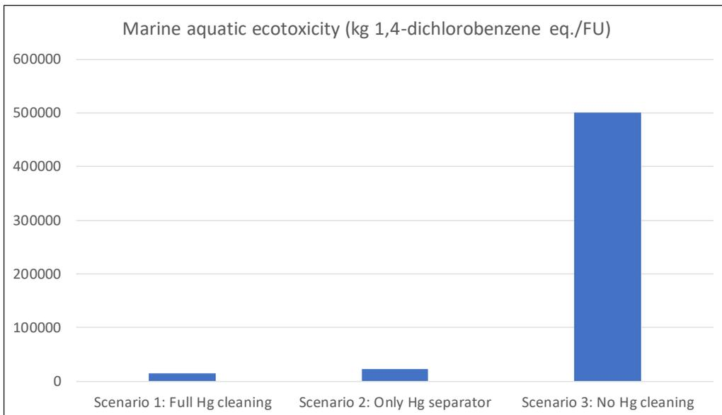
**Figure 54 Scenario comparison of the Marine aquatic ecotoxicity for the entire LCA model systems.**
