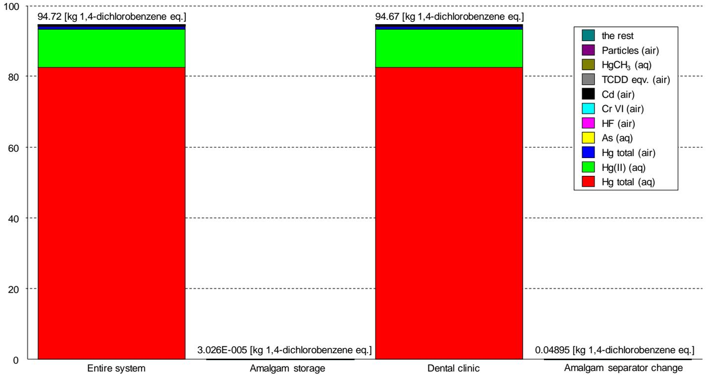
Figure 30 Human toxicity values from the entire LCA system and divided in Dental clinic, Amalgam storage, and Amalgam separator change and expressed in kg 1,4-dichlorobenzene equivalents per functional unit. The functional unit is one dentist's chair for one year of operation (226 working days). Scenario 2: with only amalgam separation and final storage of amalgam.
