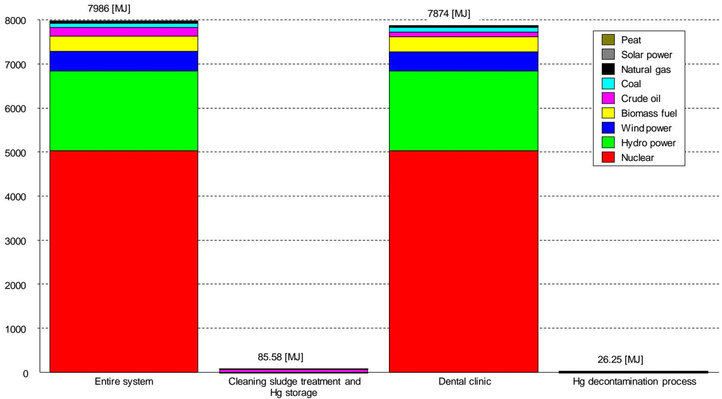
Figure 14 Use of primary energy resources from the entire LCA system and divided in Dental clinic, Cleaning sludge treatment and Hg storage, and Hg decontamination process and expressed in MJ per functional unit. The functional unit is one dentist's chair for one year of operation (226 working days). Scenario 1: with Hg decontamination, Hg processing, and final Hg storage.
