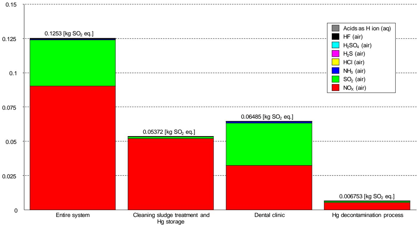
Figure 17 Acidification potential (AP) from the entire LCA system and divided in Dental clinic, Cleaning sludge treatment and Hg storage, and Hg decontamination process and expressed in kg SO<sub>2</sub> equivalents per functional unit. The functional unit is one dentist's chair for one year of operation (226 working days). Scenario 1: with Hg decontamination, Hg processing, and final Hg storage.
