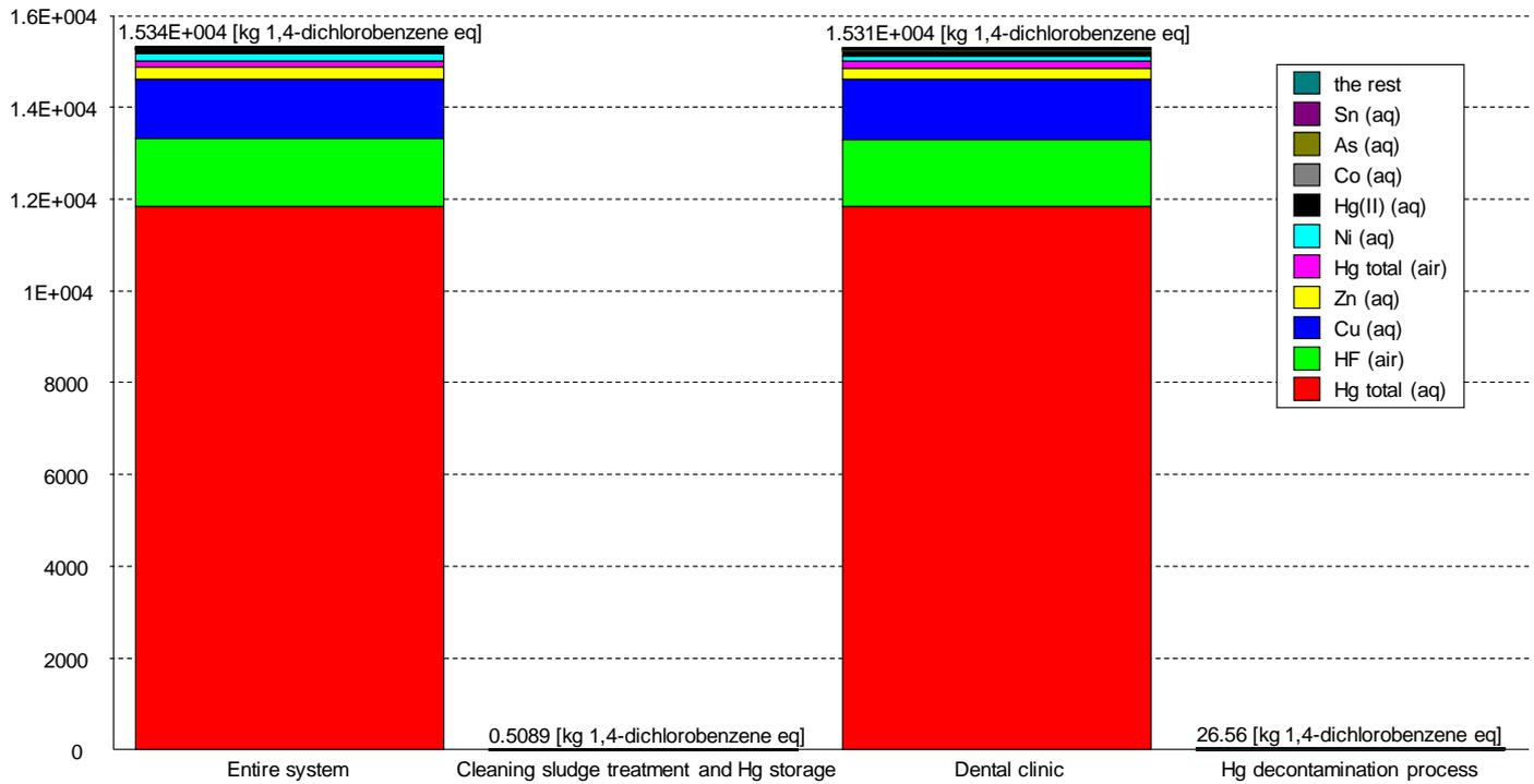
Figure 21 Marine aquatic ecotoxicity values from the entire LCA system and divided in Dental clinic, Cleaning sludge treatment and Hg storage, and Hg decontamination process and expressed in kg 1,4-dichlorobenzene equivalents per functional unit. The functional unit is one dentist's chair for one year of operation (226 working days). Scenario 1: with Hg decontamination, Hg processing, and final Hg storage.
