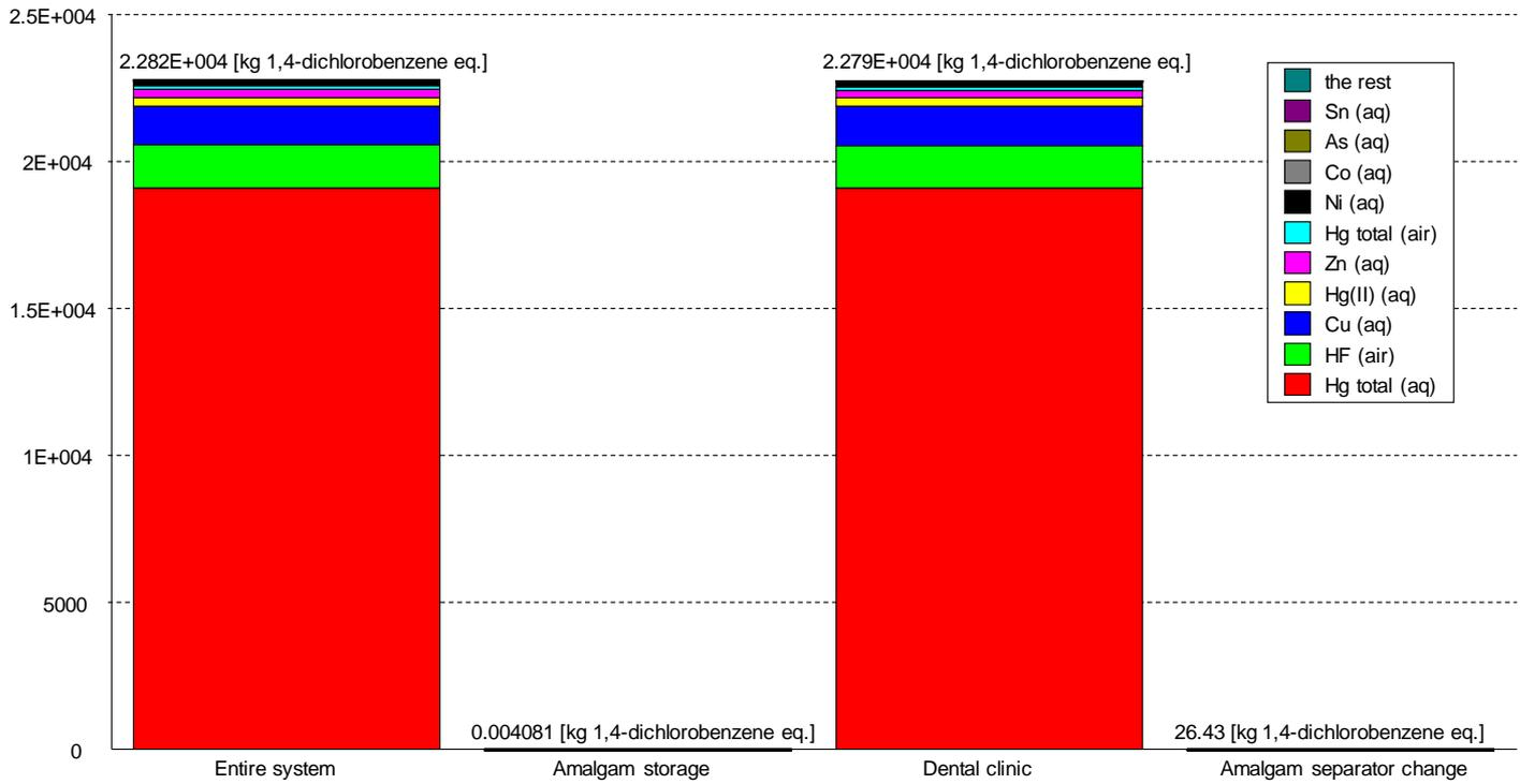
Figure 32 Marine aquatic ecotoxicity values from the entire LCA system and divided in Dental clinic, Amalgam storage, and Amalgam separator change and expressed in kg 1,4-dichlorobenzene equivalents per functional unit. The functional unit is one dentist's chair for one year of operation (226 working days). Scenario 2: with only amalgam separation and final storage of amalgam.
