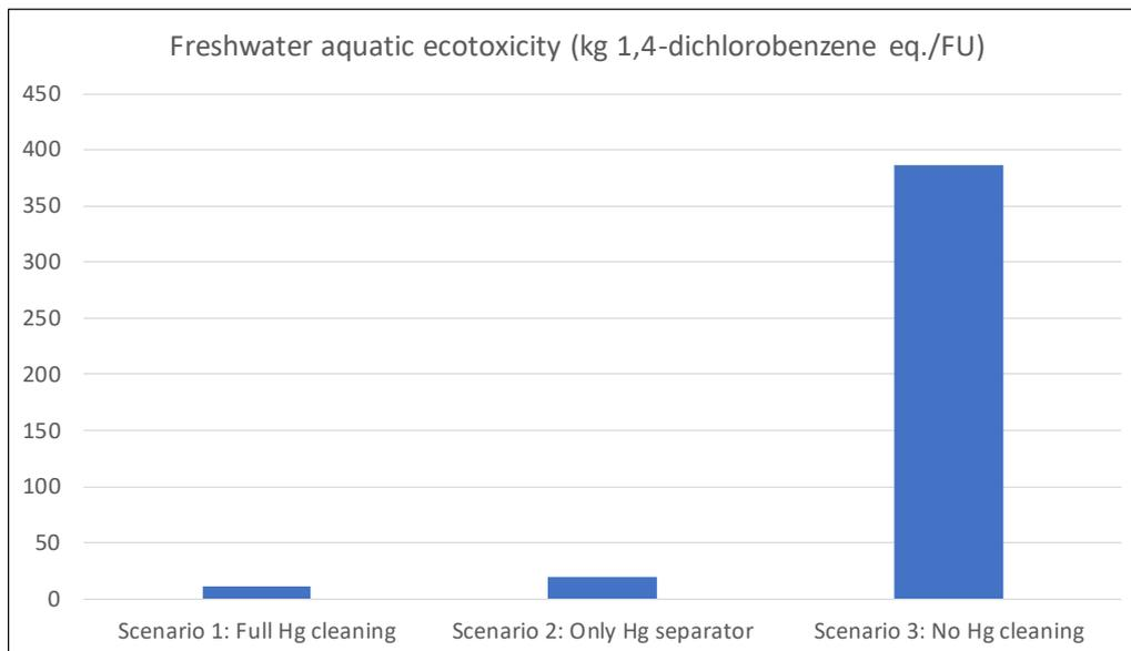
**Figure 55 Scenario comparison of the Freshwater aquatic ecotoxicity for the entire LCA model systems.**
