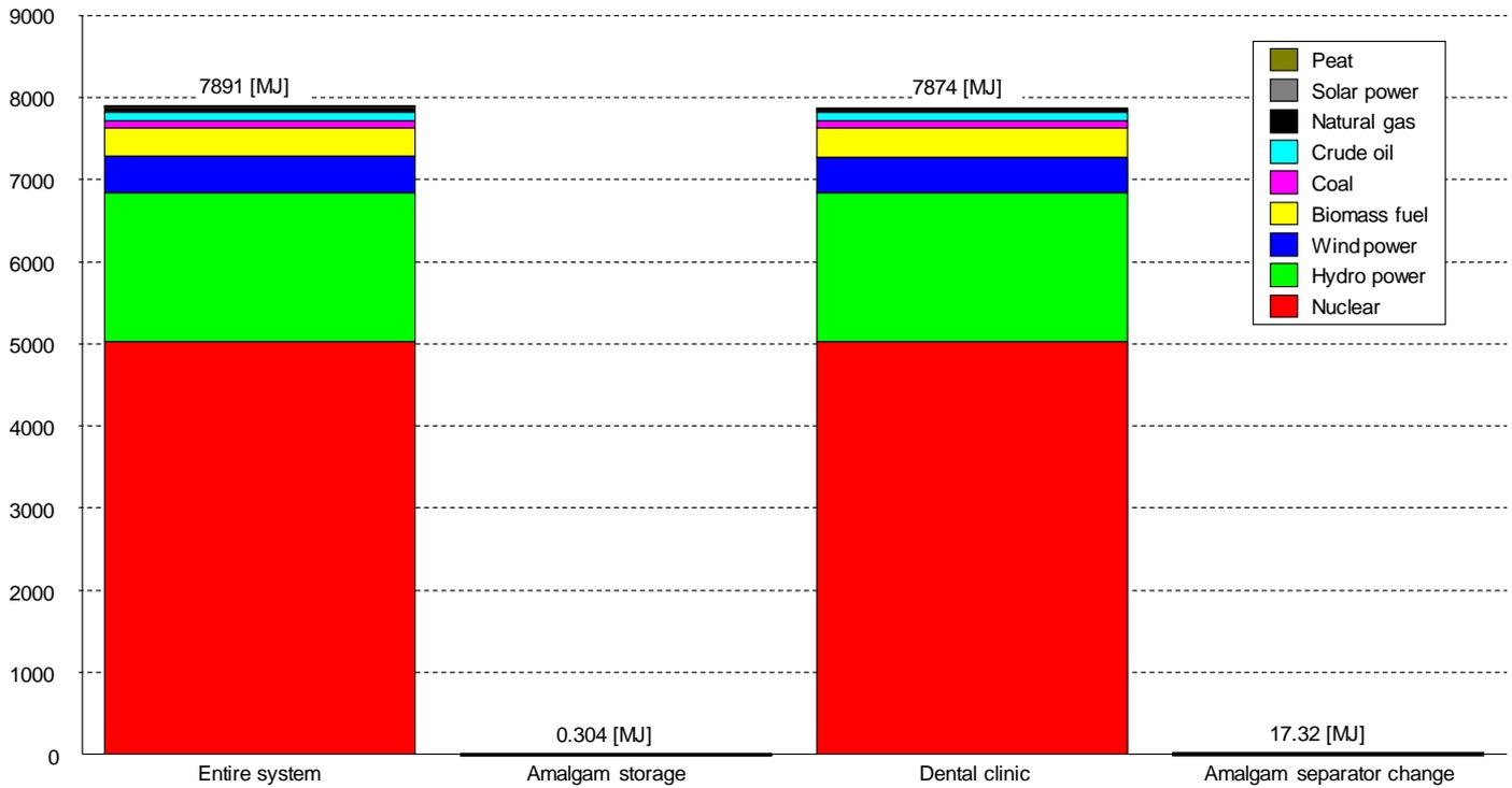
Figure 25 Use of primary energy resources from the entire LCA system and divided in Dental clinic, Amalgam storage, and Amalgam separator change and expressed in MJ per functional unit. The functional unit is one dentist's chair for one year of operation (226 working days). Scenario 2: with only amalgam separation and final storage of amalgam.
