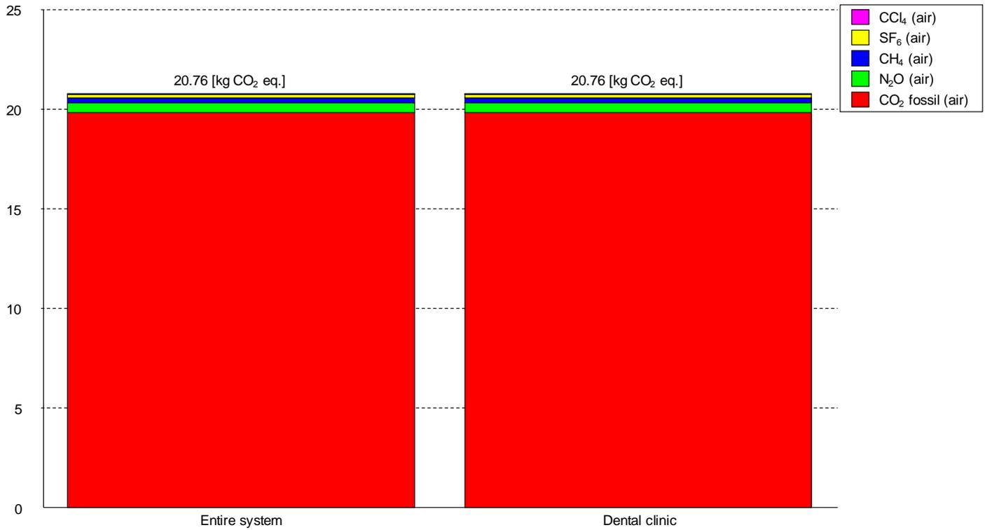
Figure 37 Global warming potential (GWP 100) from the entire LCA system including only the Dental clinic without Hg/amalgam separation and expressed in kg CO<sub>2</sub> equivalents per functional unit. The functional unit is one dentist's chair for one year of operation (226 working days). Scenario 3: with no mercury or amalgam separation or handling, all to recipient.
