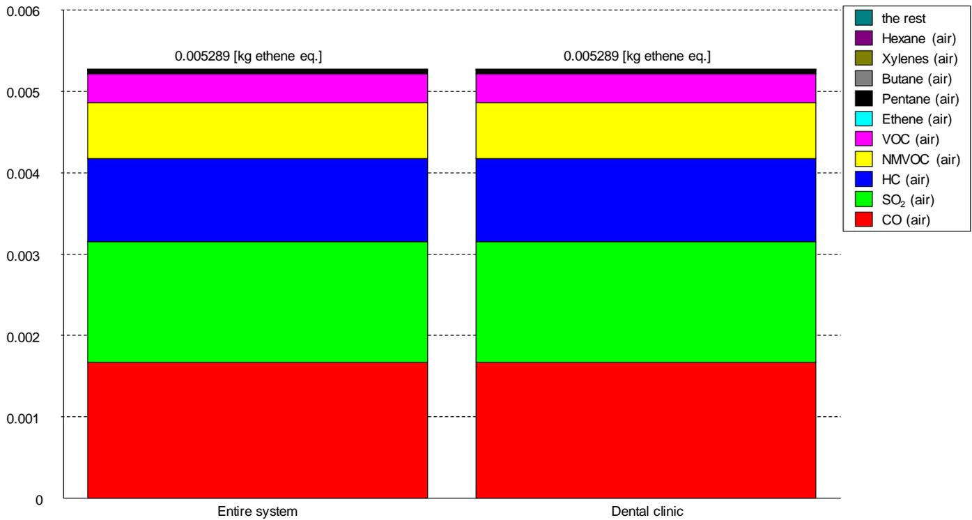
Figure 40 Photochemical ozone creation potentials (POCP) from the entire LCA system including only the Dental clinic without Hg/amalgam separation and expressed in kg ethene equivalents per functional unit. The functional unit is one dentist's chair for one year of operation (226 working days). Scenario 3: with no mercury or amalgam separation or handling, all to recipient.
