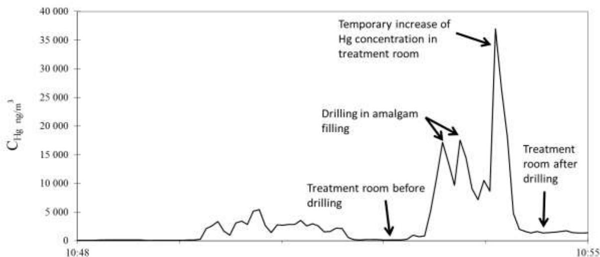
**Figure 11** Hg(0) concentrations in air measured before, during and after drilling of an amalgam filling (not on a patient) measured with the Lumex RA-915+ instrument.
