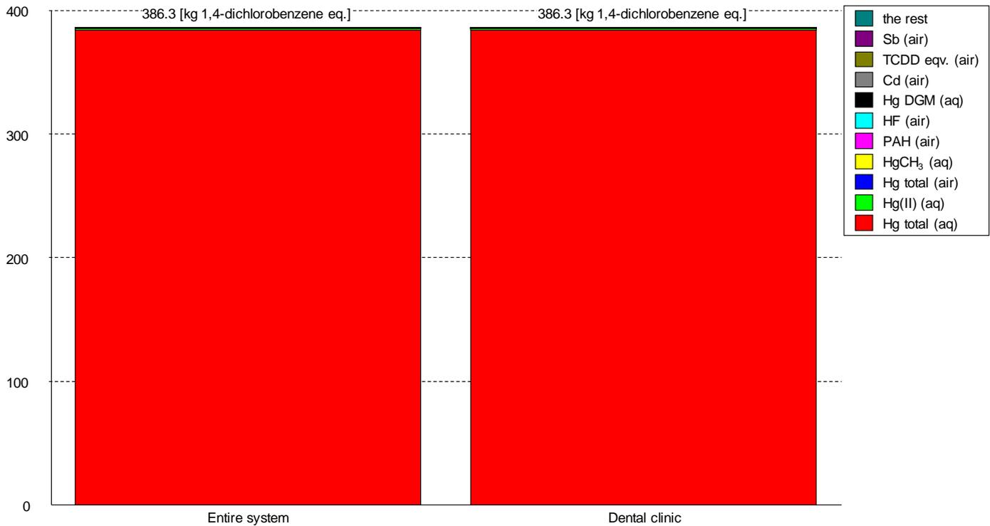
Figure 44 Freshwater aquatic ecotoxicity values from the entire LCA system including only the Dental clinic without Hg/amalgam separation and expressed in kg 1,4-dichlorobenzene equivalents per functional unit. The functional unit is one dentist's chair for one year of operation (226 working days). Scenario 3: with no mercury or amalgam separation or handling, all to recipient.
