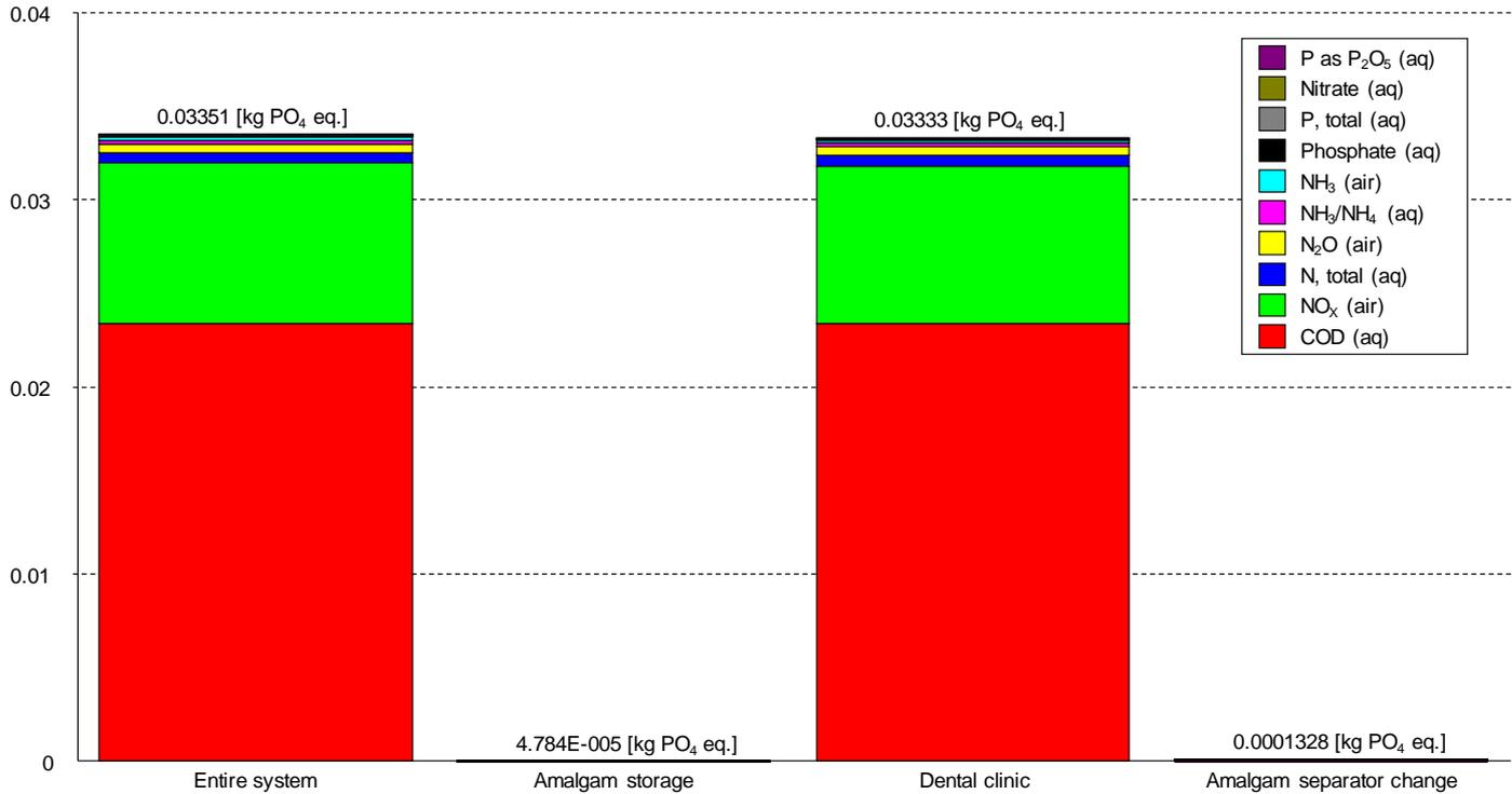
**Figure 27** Eutrophication potential (EP) from the entire LCA system and divided in Dental clinic, Amalgam storage, and Amalgam separator change and expressed in kg PO<sub>4</sub><sup>3-</sup> equivalents per functional unit. The functional unit is one dentist's chair for one year of operation (226 working days). Scenario 2: with only amalgam separation and final storage of amalgam.
