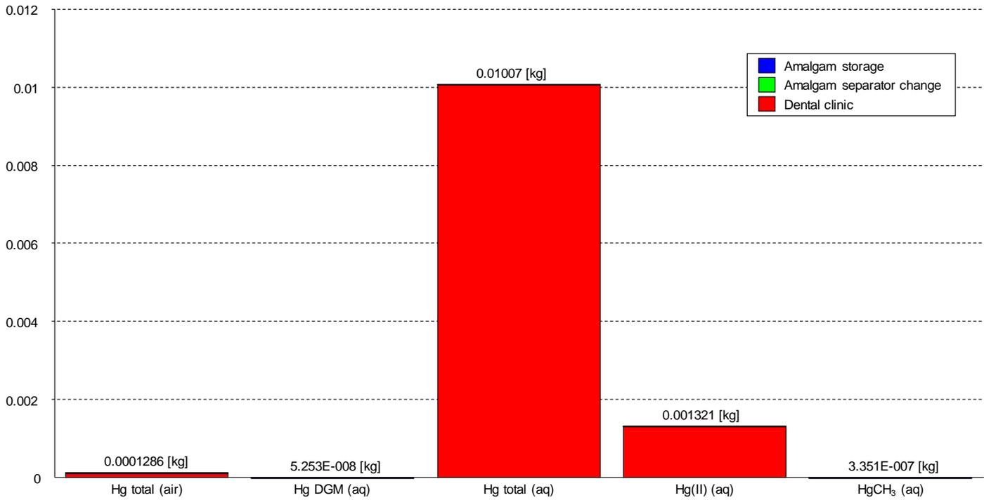
**Figure 24** Total Hg emissions from the entire LCA system expressed in kg per functional unit. The functional unit is one dentist's chair for one year of operation (226 working days). Scenario 2: with only amalgam separation and final storage of amalgam.
