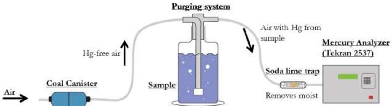
**Figure 4** Principle of purging gaseous Hg(0), or DGM, in water samples for analysis. A Lumex RA-915+ mercury analyzer was used for analysis (not a Tekran 2537 as shown in this picture) (Nerentorp Mastromonaco, 2016).
