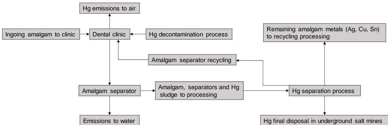
**Figure 1** Schematic figure over the technical system for Hg separation at dental clinics in Sweden.
