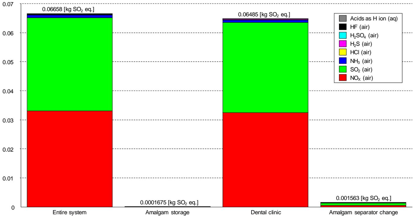
Figure 28 Acidification potential (AP) from the entire LCA system and divided in Dental clinic, Amalgam storage, and Amalgam separator change and expressed in kg SO<sub>2</sub> equivalents per functional unit. The functional unit is one dentist's chair for one year of operation (226 working days). Scenario 2: with only amalgam separation and final storage of amalgam.
