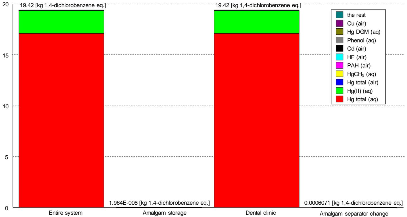
Figure 33 Freshwater aquatic ecotoxicity values from the entire LCA system and divided in Dental clinic, Amalgam storage, and Amalgam separator change and expressed in kg 1,4-dichlorobenzene equivalents per functional unit. The functional unit is one dentist's chair for one year of operation (226 working days). Scenario 2: with only amalgam separation and final storage of amalgam.
