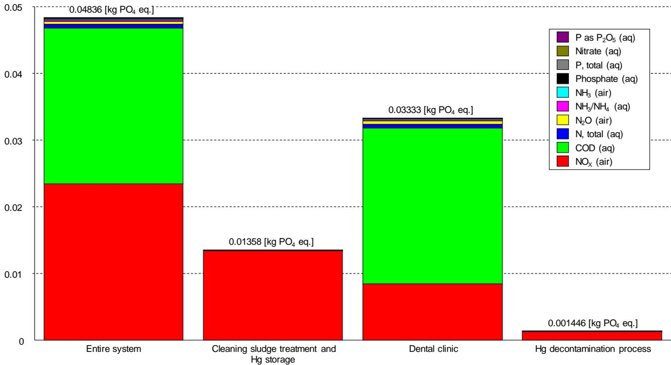
Figure 16 Eutrophication potential (EP) from the entire LCA system and divided in Dental clinic, Cleaning sludge treatment and Hg storage, and Hg decontamination process and expressed in kg PO<sub>4</sub><sup>3-</sup> equivalents per functional unit. The functional unit is one dentist's chair for one year of operation (226 working days). Scenario 1: with Hg decontamination, Hg processing, and final Hg storage.
