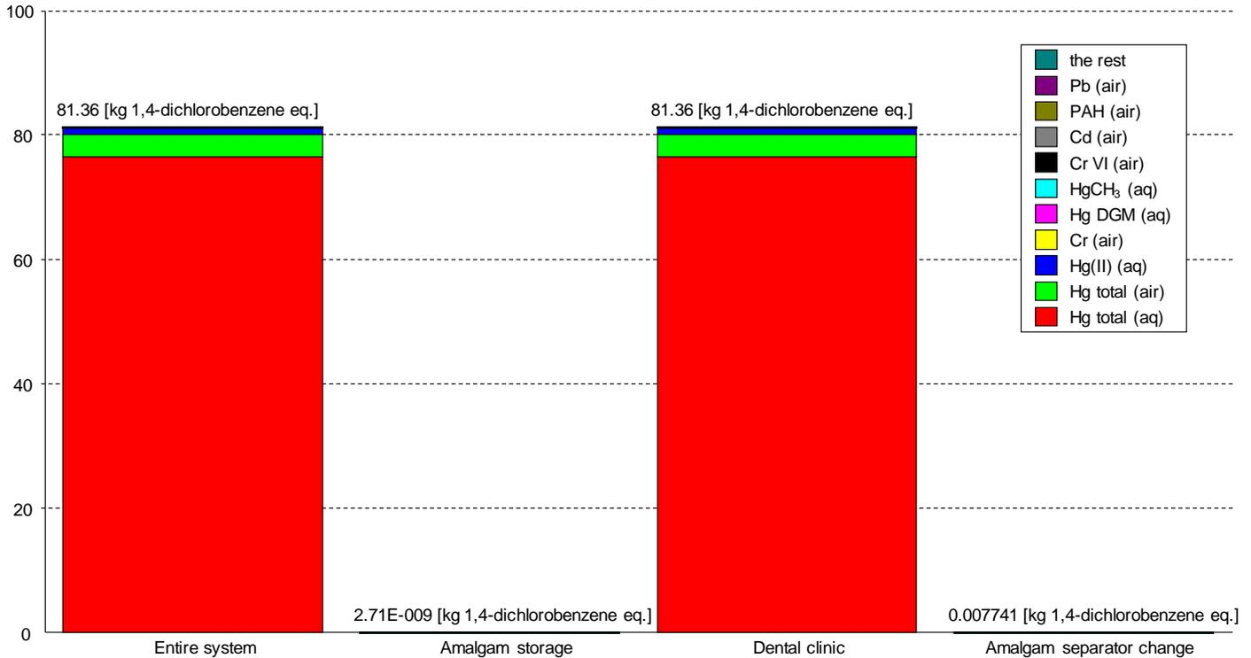
Figure 31 Terrestrial ecotoxicity values from the entire LCA system and divided in Dental clinic, Amalgam storage, and Amalgam separator change and expressed in kg 1,4-dichlorobenzene equivalents per functional unit. The functional unit is one dentist's chair for one year of operation (226 working days). Scenario 2: with only amalgam separation and final storage of amalgam.
