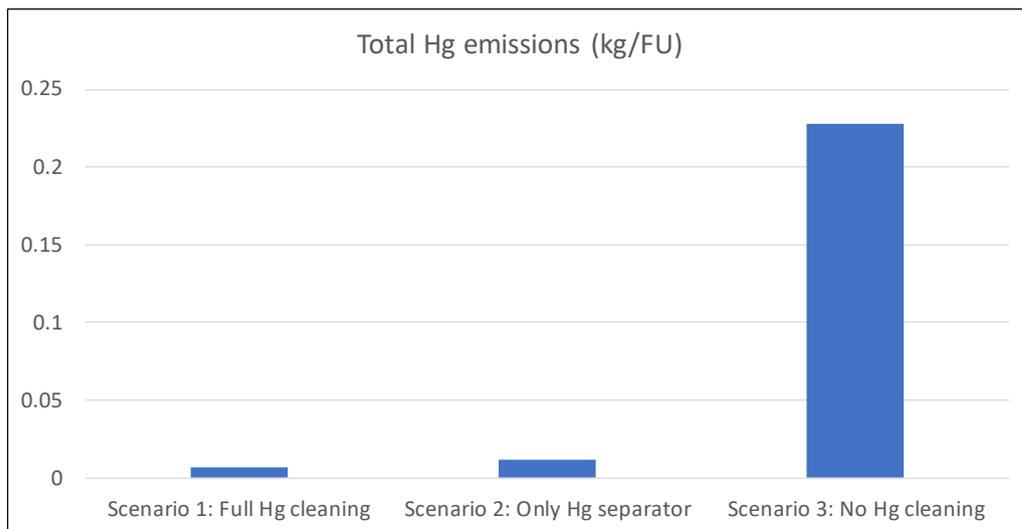
**Figure 47 Scenario comparison of the total Hg emissions from the entire LCA model systems.**
