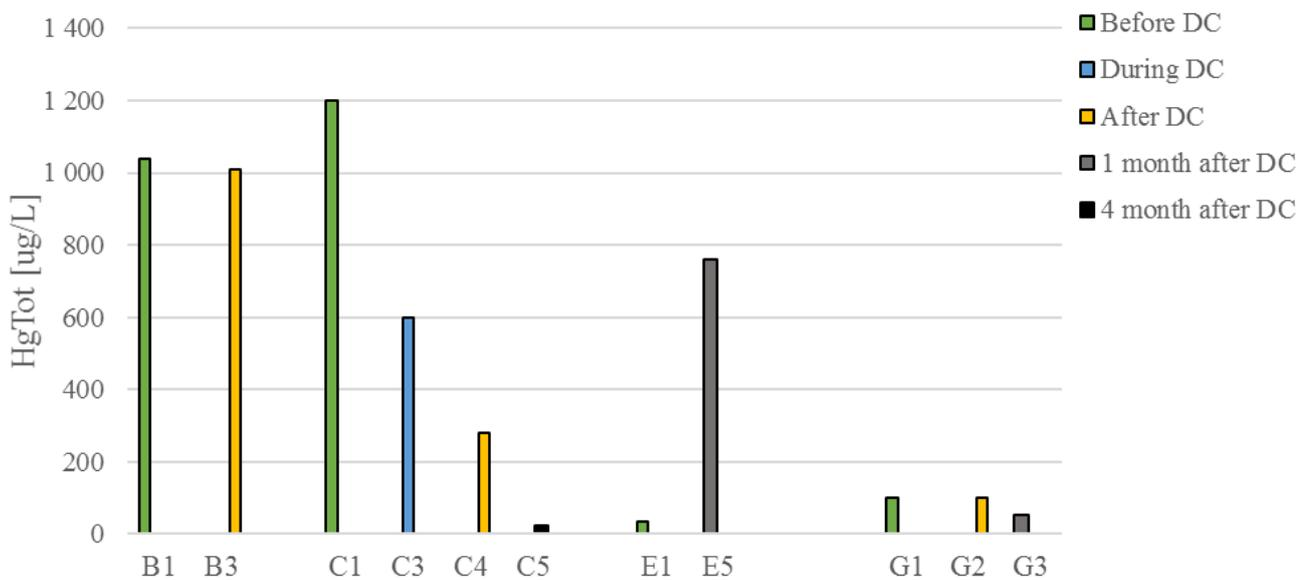
**Figure 9** HgTot concentrations in IVL samples taken before, during and after the decontamination process (DC). Compared to Hg concentrations in water sampled one or four months after DC.
