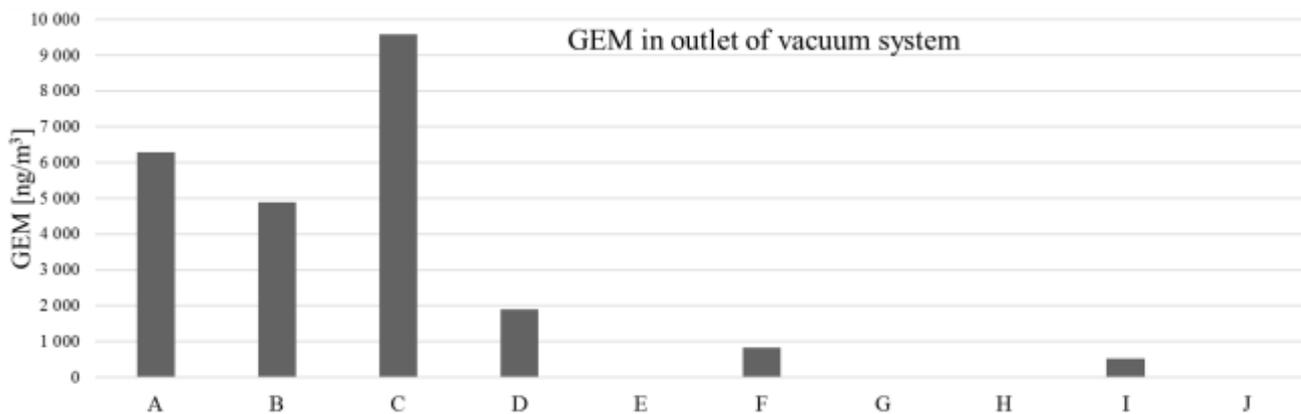
**Figure 7** Average GEM concentrations measured at the outlet of the vacuum system, at dental clinic A, B, C, D, F and I, before decontamination.
