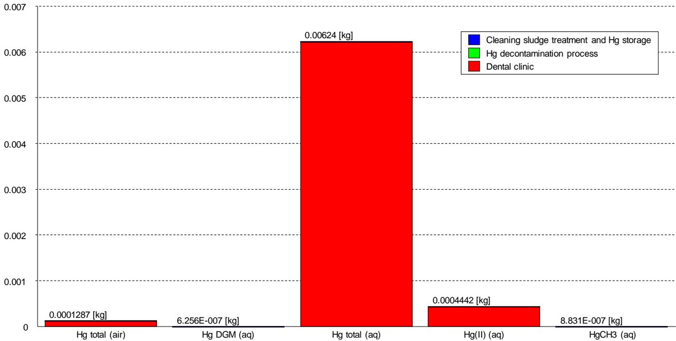
**Figure 13** Total Hg emissions from the entire LCA system expressed in kg per functional unit. The functional unit is one dentist's chair for one year of operation (226 working days). Scenario 1: with Hg decontamination, Hg processing, and final Hg storage.
