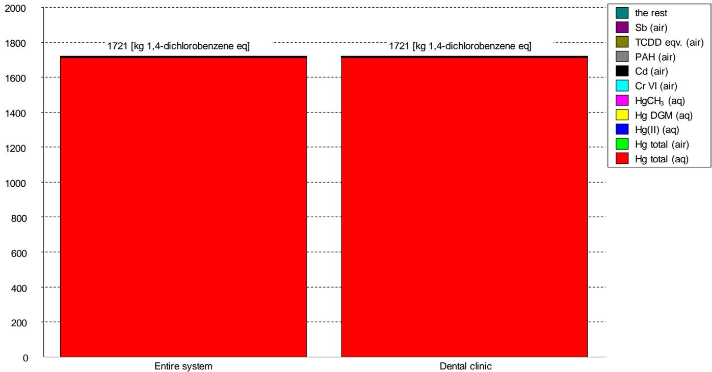
Figure 42 Terrestrial ecotoxicity values from the entire LCA system including only the Dental clinic without Hg/amalgam separation and expressed in kg 1,4-dichlorobenzene equivalents per functional unit. The functional unit is one dentist's chair for one year of operation (226 working days). Scenario 3: with no mercury or amalgam separation or handling, all to recipient.
