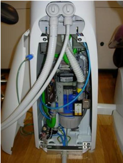
*Example of a dry suction system with centrifuging dental amalgam separator*
